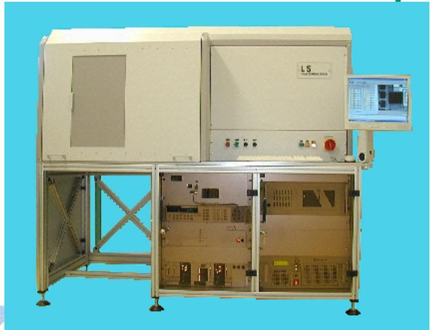
**LS9000TD** thick-film trimmers are mounted on a profile frame. Personal computer, laser power supply, motor control and measuring instruments are embedded within the frame. The whole front side of the work station can be lifted for set-up (change of probe cards). The housing is already prepared for a later adaption of loader units.
